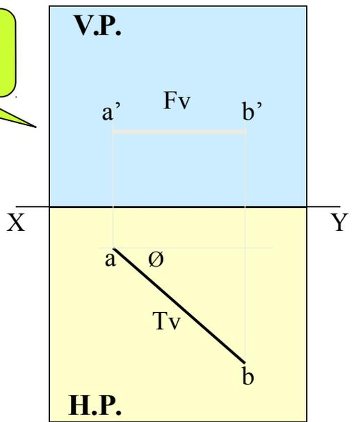
5. A Line inclined to both Hp and Vp
