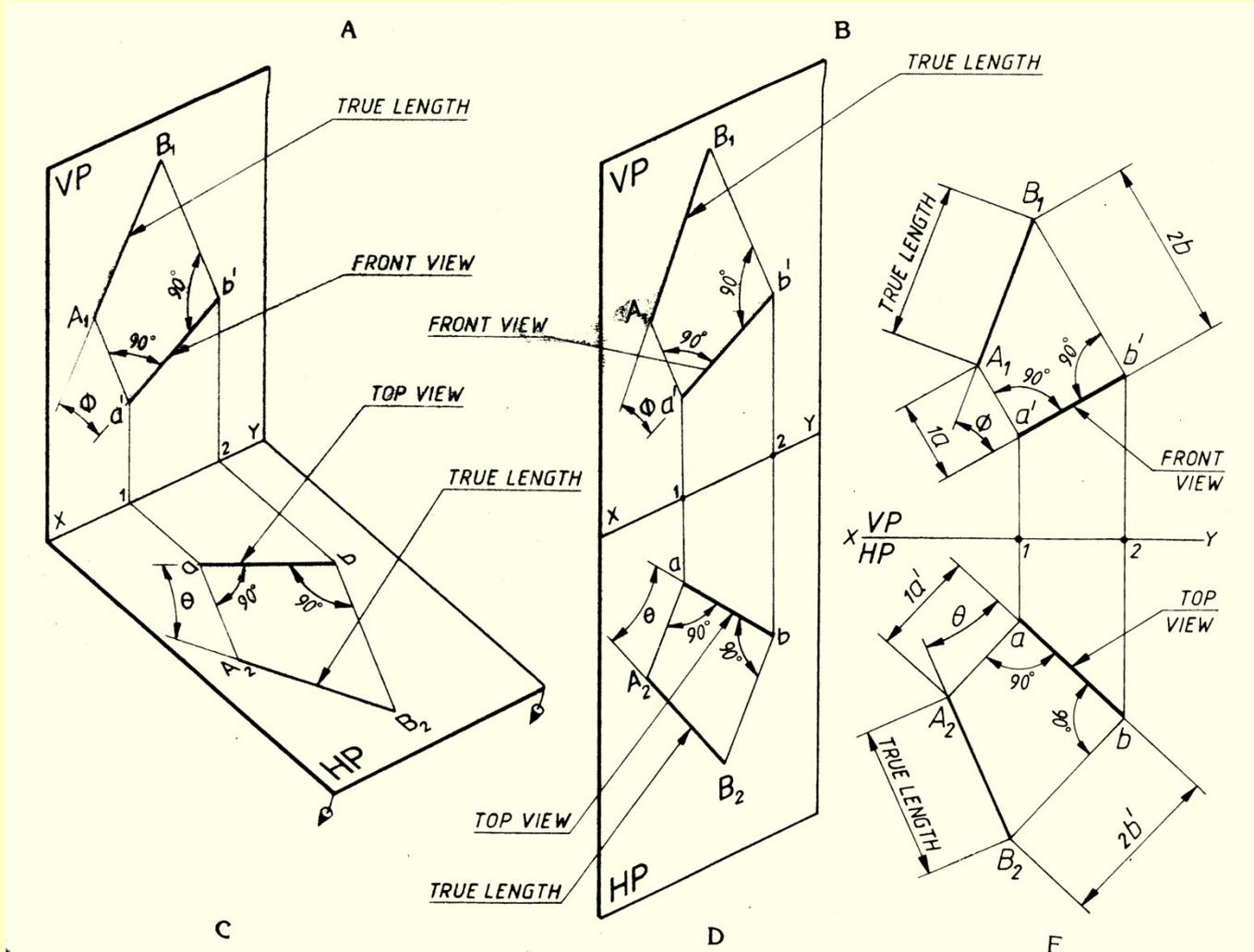
**(13) The front view of the line AB of length 70 mm is inclined at  $30^\circ$  to xy line and measures 45 mm. The end A is 20 mm above HP and 25 mm in front of VP. Draw the projections of the line and find the inclinations with HP and VP by i) rotating line method and ii) trapezoidal method.**
