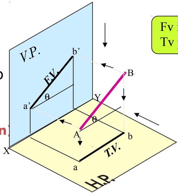
Fv inclined to xy
