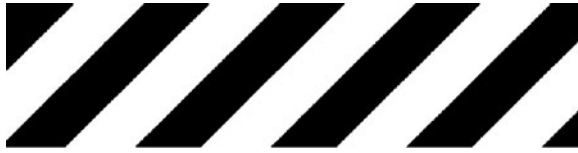
FIGURE 8-36 Taxiway ending marker.
