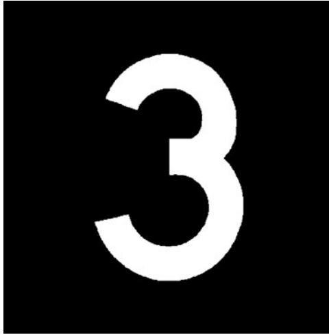
FIGURE 8-29 Runway distance remaining sign.
