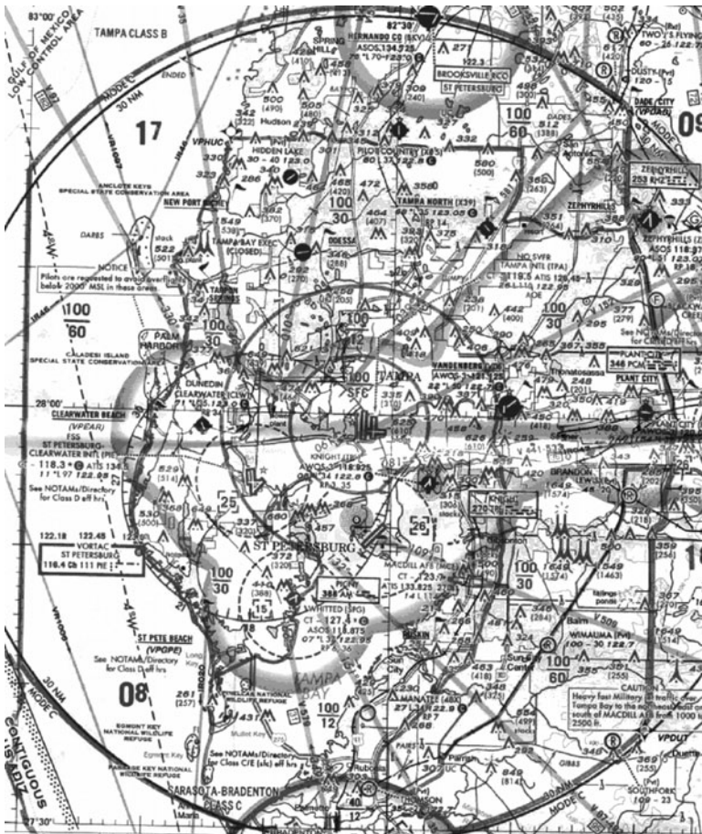
FIGURE 3-3 Class B airspace around Tampa International Airport, Tampa, Florida.
