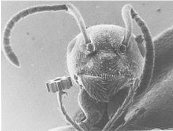
SEM picture of an ant carrying a LIGA micro gear
