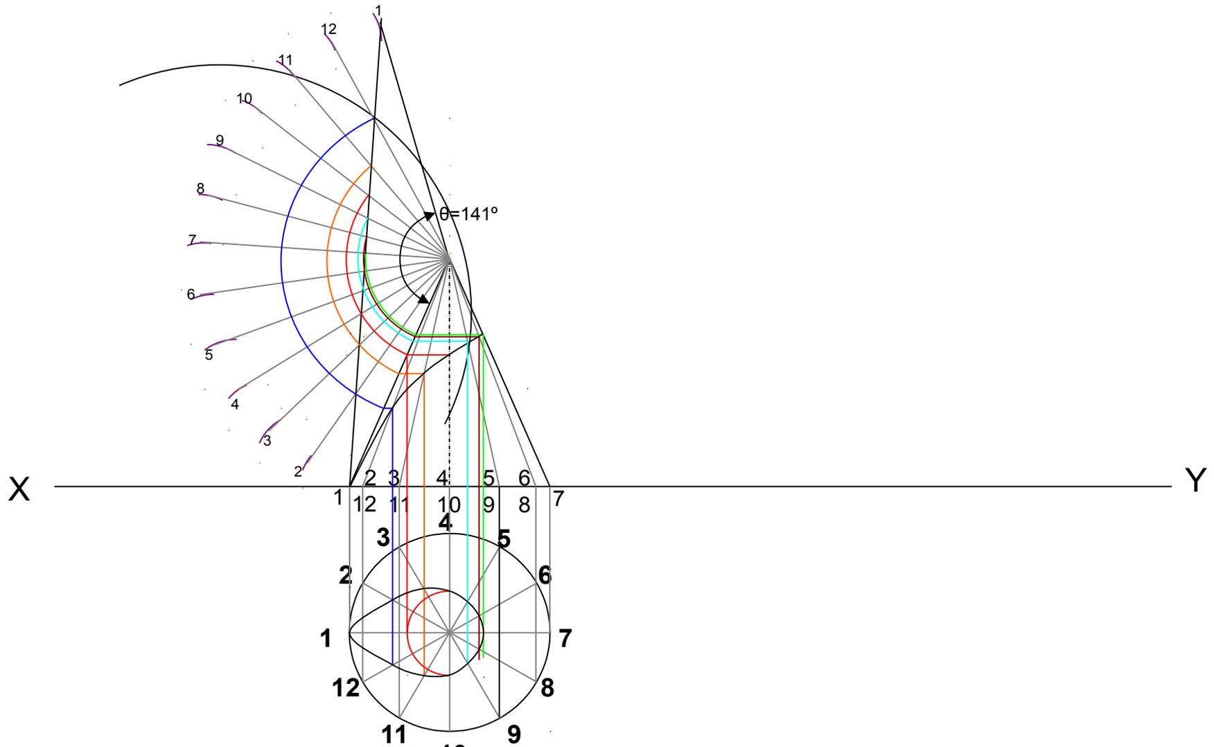
Q 15.26: A right circular cone base 30 mm side and height 50 mm rests on its base on H.P. It is cut by a section plane perpendicular to the V.P., inclined at  $45^\circ$  to the H.P. and bisecting the axis. Draw the projections of the truncated cone and develop its lateral surface.
