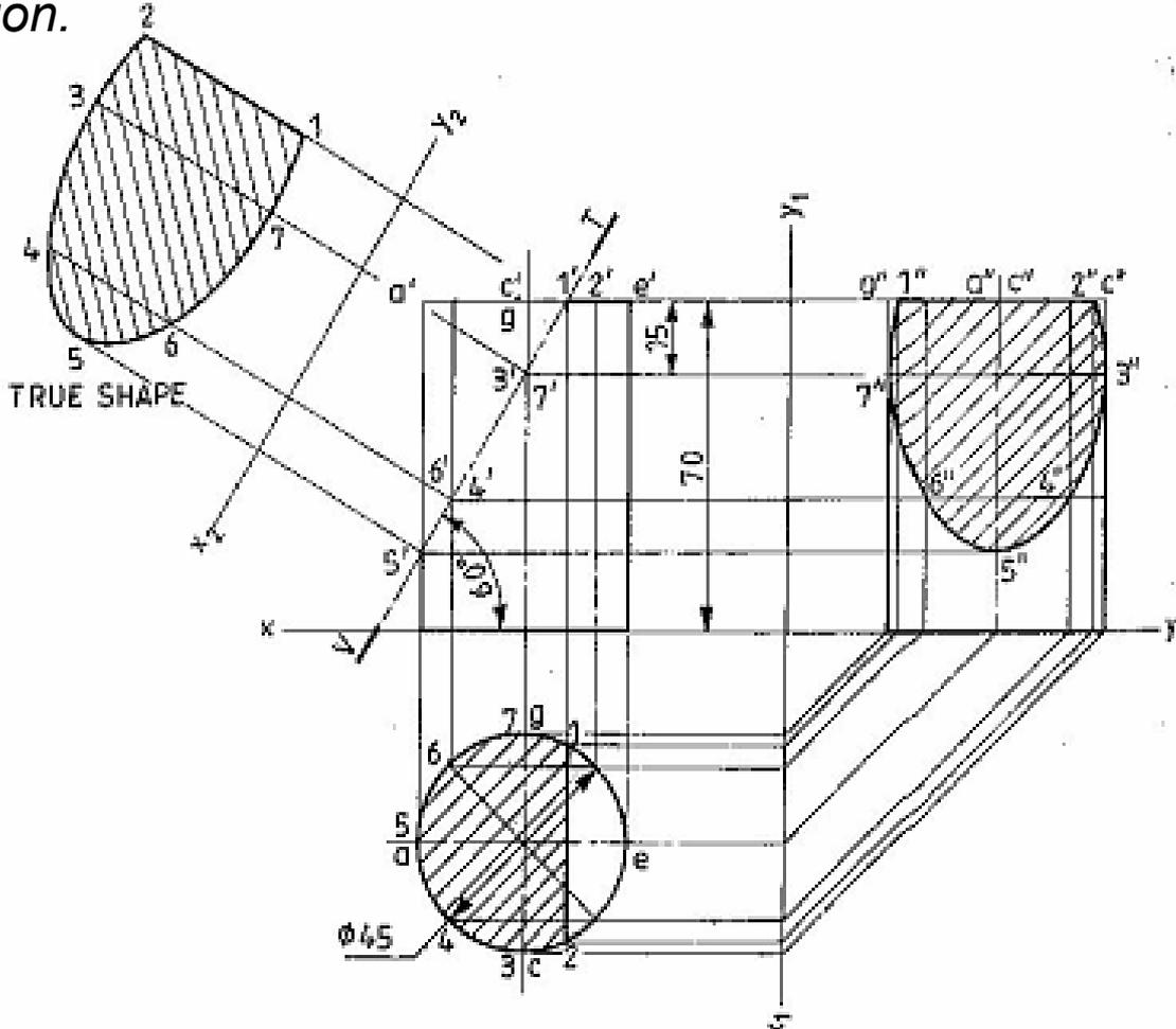
**Note:** true shape of a section: when the section plane is inclined, the section has to be projected on an auxiliary plane, parallel to the cutting plane, to obtain its true shape.
