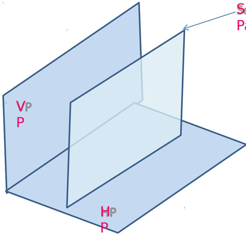
Section plane perpendicular to HP and Parallel to VP
