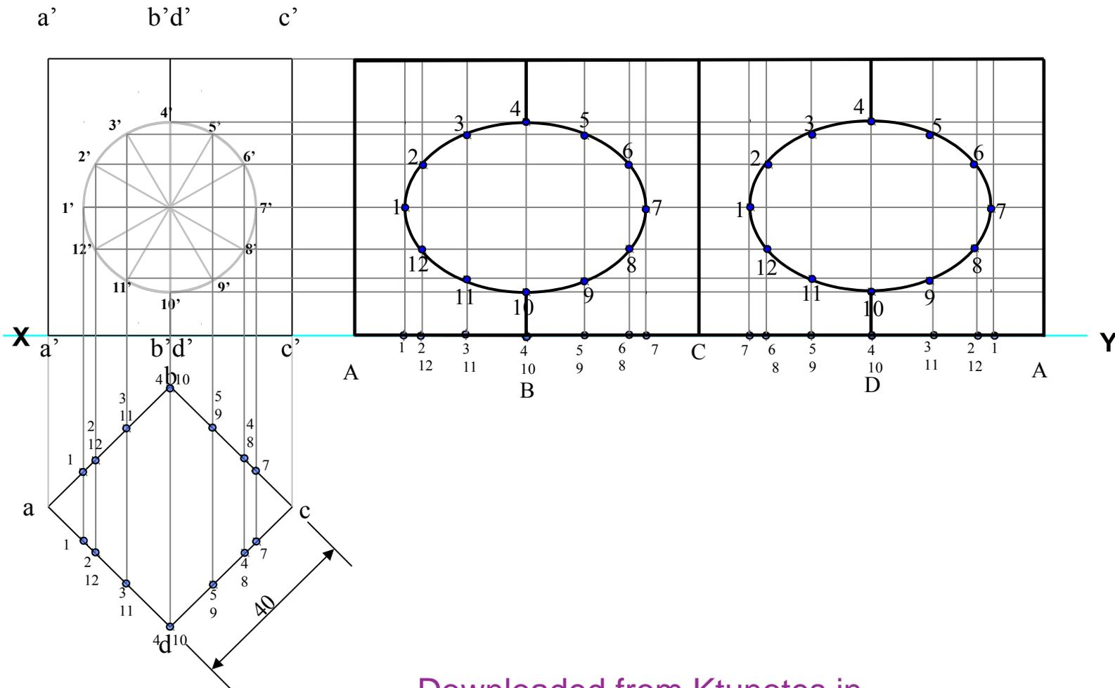
**Q.15.11: A right circular cylinder, base 50 mm diameter and axis 60 mm long, is standing on HP on its base. It has a square hole of size 25 in it. The axis of the hole bisects the axis of the cylinder and is perpendicular to the VP. The faces of the square hole are equally inclined with the HP. Draw its projections and develop lateral surface of the cylinder.**
