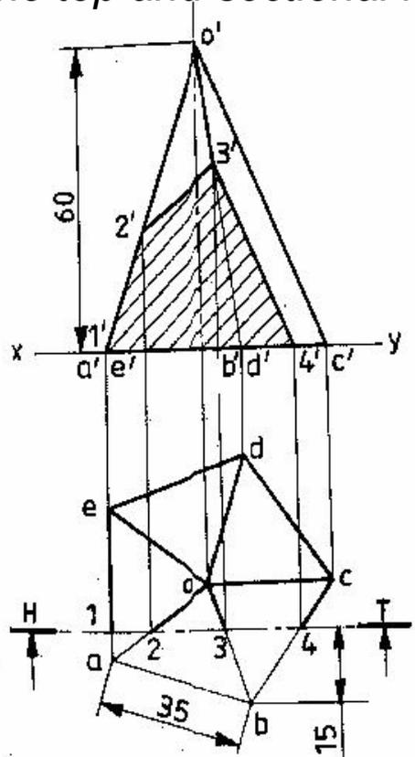
**NOTE:** True shape of a section: the projection of the section on a plane parallel to the section plane, will appear in its true shape of the section. Thus, when the section plane is parallel to H.P, the true shape of the section will be seen in the sectional top view. When it is parallel to V.P, the true shape of the section will appear in the sectional front view.
