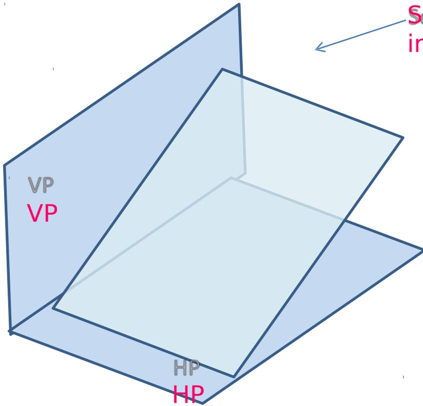
Section plane perpendicular to VP and inclined to HP
