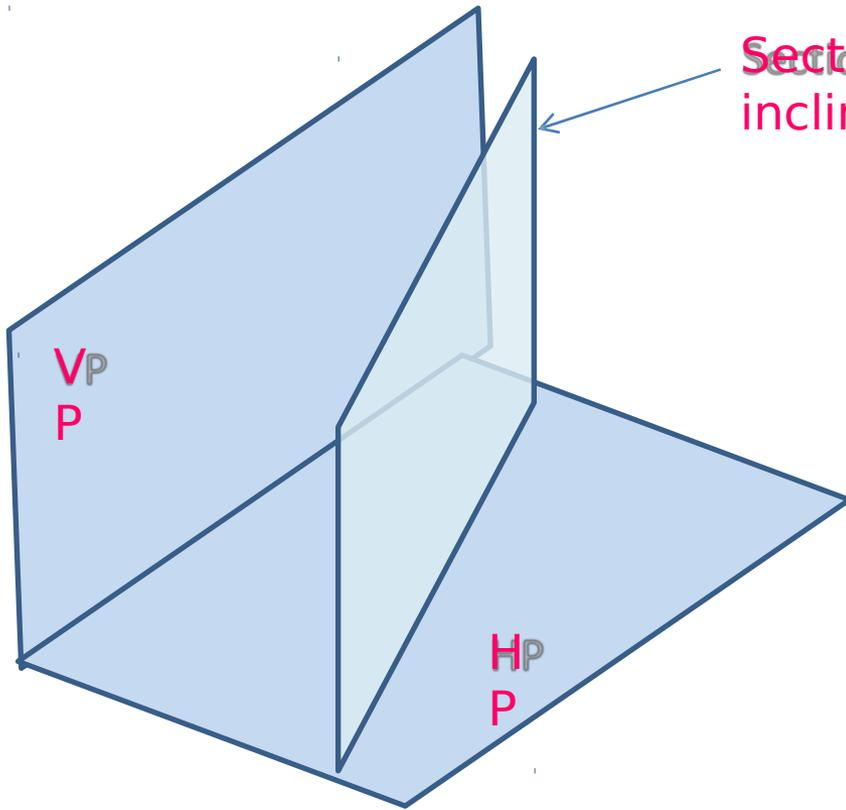
Section plane perpendicular to HP and inclined to VP
