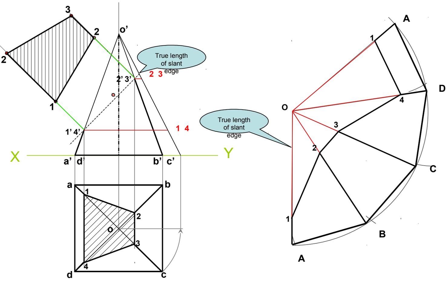
Q 14.11: A square pyramid, base 40 mm side and axis 65 mm long, has its base on the HP and all the edges of the base equally inclined to the VP. It is cut by a section plane, perpendicular to the VP, inclined at  $45^\circ$  to the HP and bisecting the axis. Draw its sectional top view, sectional side view and true shape of the section. Also draw its development.
