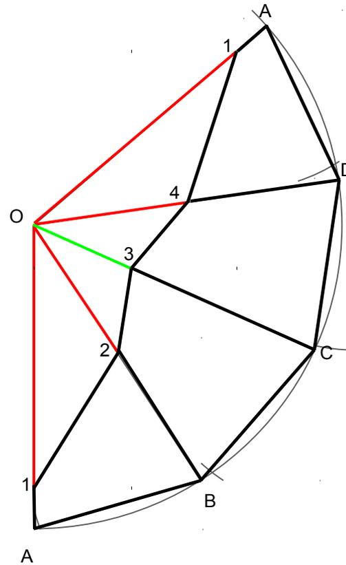
Q 15.26: draw the projections of a cone resting on the ground on its base and show on them, the shortest path by which a point P, starting from a point on the circumference of the base and moving around the cone will return to the same point. Base of cone 65 mm diameter ; axis 75 mm long.
