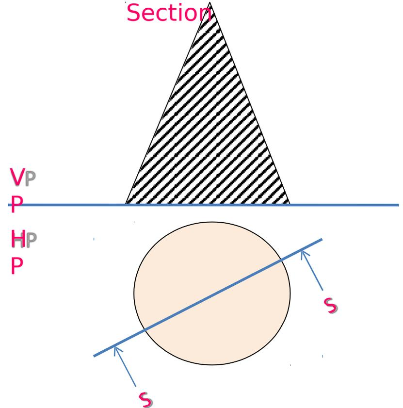
Section plane perpendicular to HP and inclined to VP
